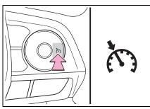
2 Accelerate or decelerate, with accelerator pedal operation, to the desired speed (at or above approximately 30 km/h [20 mph]) and press the "-SET" switch to set the speed.
