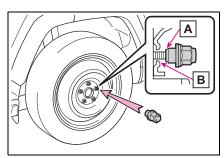
When replacing an aluminum wheel with an aluminum wheel, turn the wheel nuts until the washers  $\boxed{\mathbf{A}}$  come into
