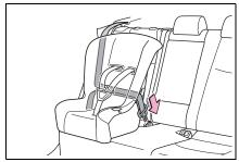
5 If your child restraint system is not equipped with a lock-off (a seat belt locking feature), secure the child restraint system using a locking clip.
