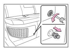
3 Remove the air intake vent cover.
