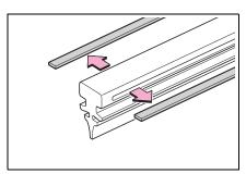
4 Insert the wiper insert starting from the claw at the center of the wiper blade. Pass the wiper insert through the 3 claws so that it sticks out from the stopper, and then pass the wiper insert through the final remaining claw.
