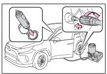
**21** Turn the compressor switch on and wait for several seconds,
