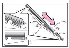
When installing a wiper blade, reverse the procedure in step 1.
