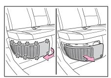
**4** Remove the air intake vent filter. Disengage the 4 center claws from the
