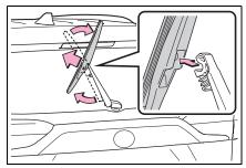
Pull the wiper insert out past the stopper on the wiper blade, and then continue to pull until it is completely removed.
