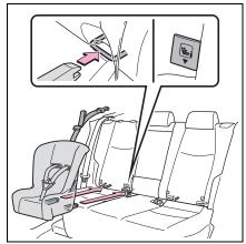
**4** After installing the child restraint system, rock it back and forth to ensure that it is installed securely. (→P.63)
