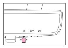
2 Press or to enable (ON)/disable (OFF) the automatic anti-glare function.
