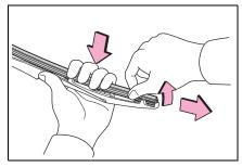
Remove the 2 metal plates from the old wiper insert and install
