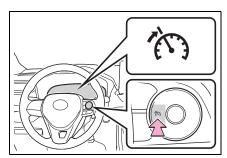
2 Accelerate or decelerate, with accelerator pedal operation, to the desired maximum speed and press the "-SET" switch to set the speed.
