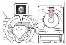
When the current set speed is higher than the recognized speed limit
