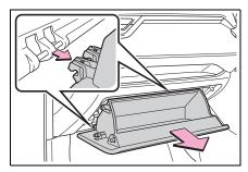
5 Unlock the filter cover (A), pull the filter cover out of the claws
