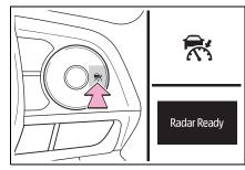
2 Accelerate or decelerate, with accelerator pedal operation, to the desired vehicle speed (at or above approximately 30 km/h [20 mph]) and press the "-SET" switch to set the speed.
