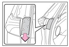
Remove the screws and remove the light unit.
