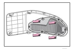
Disengage the claws in the order of A and B to remove the filter from the cover.
