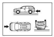
The SRS curtain shield airbags do not generally inflate if the vehicle is involved in a rear collision, if it rolls over, or if it is involved in a low-speed side or low-speed frontal collision.
