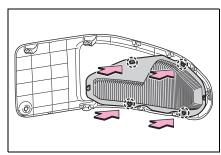
7 Install the air intake vent cover.
