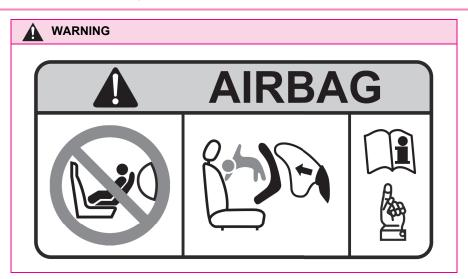
Only put a forward-facing child restraint system on the front seat when unavoidable. When installing a forward-facing child restraint on the front passenger seat, move the seat as far back as possible. Failing to do so may result in death or serious injury if the airbags deploy (inflate).
