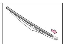
5 Check that the wiper blade claws are fitted in the grooves of the wiper insert.
