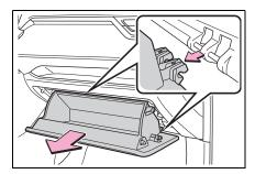
Unlock the filter cover (A), pull the filter cover out of the claws
