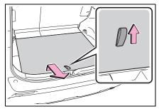
Place the deck board through the groove and move forward.
