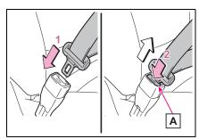
To fasten the seat belt, push the plate into the buckle until a click sound is heard.
