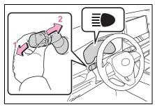
1 With the headlights on, push the lever away from you to turn on
