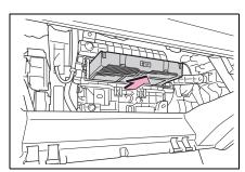
7 Remove the air conditioning filter and replace it with a new one.
