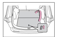
Place the edge into the groove (A), and with the deck board in a standing state, put the edge into the holes (B).
