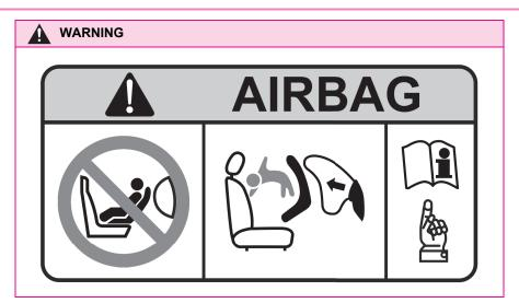
Only put a forward-facing child restraint system on the front seat when unavoidable. When installing a forward-facing child restraint on the front passenger seat, move the seat as far back as possible. Failing to do so may result in death or serious injury if the airbags deploy (inflate).
