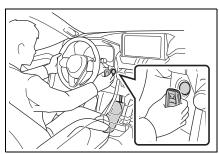
3 Firmly depress the brake pedal and check that a is displayed on the multi-information display. **4** Press the power switch shortly and firmly.
