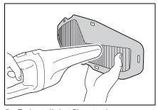
6 Reinstall the filter to the cover.
