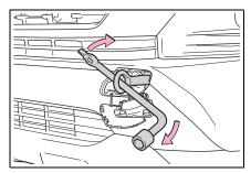
Securely attach cables or chains to the towing eyelet.
