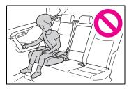
When a junior seat is installed, always ensure that the shoulder belt is positioned across the center of the child's shoulder. The belt should be kept away from the child's neck, but not so that it could fall off the child's shoulder.
