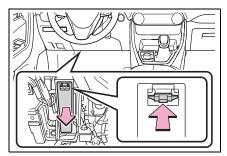
Right-hand drive vehicles: Push the tab in and remove the cover, and then remove the lid.
