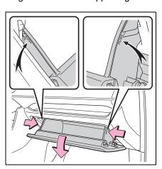
4 With the glove box fully open, slightly lift up the glove box and pull toward the seat to detach the bottom of the glove box.
