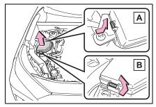
► Engine compartment: Type B fuse box
