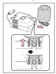
**4** Connect the hose to the bottle. Make sure to insert the hose until its
