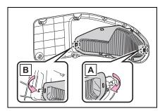
Engage the 4 center claws to install the filter.
