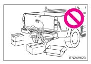
• Do not place flammable materials near the exhaust pipe.
