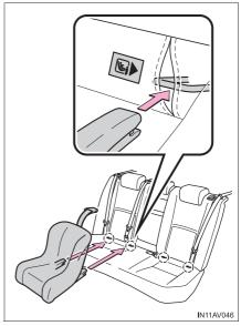
After installing the child restraint system, rock it back and forth to ensure that it is installed securely.  $(\rightarrow P. 68)$
