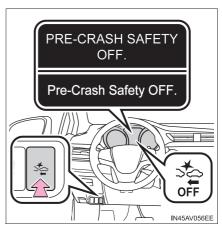
Vehicles with a smart entry & start system: The system is enabled each time the engine switch is turned to IGNITION ON mode.
