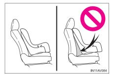
If the seat belt shoulder anchor is ahead of the child seat belt guide, move the seat cushion forward.
