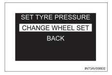
switch while the cursor is on "CHANGE" to switch to the other registered wheel set. If operation is completed, the tire pressure warning light will blink 3 times.
