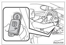
3 Press the engine switch within 10 seconds after the buzzer sounds, keeping the brake pedal (Multidrive) or clutch pedal (manual transmission) depressed.
