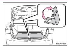
2 Secure the panel using the hook provided.
