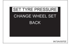
7 Press and hold the "DISP" switch while the cursor is on "SET" to initialize the system. If initialization is completed, the tire pressure warning light will blink 3 times.
